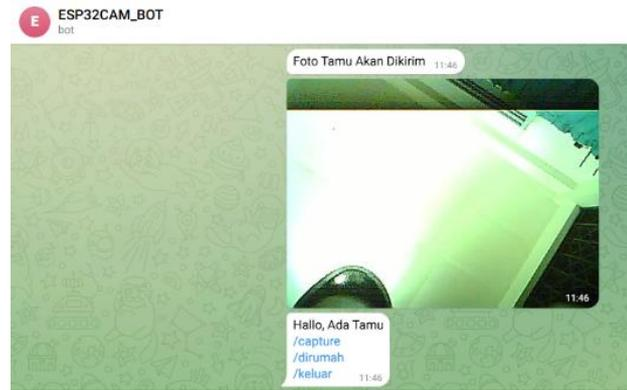
Figure 3 : Testing process showing image capture and Telegram notification
