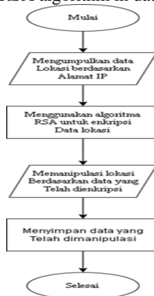
Figure 3. Flowchart of RSA algorithm implementation on data encryption
